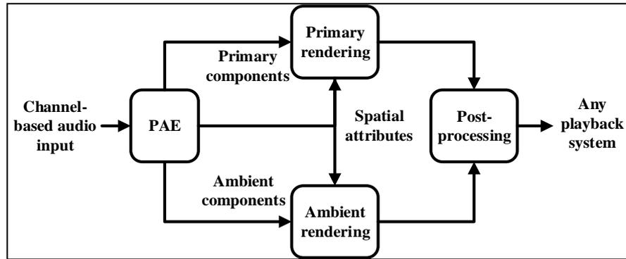
Figure 1 Block diagram of PAE based spatial audio reproduction
