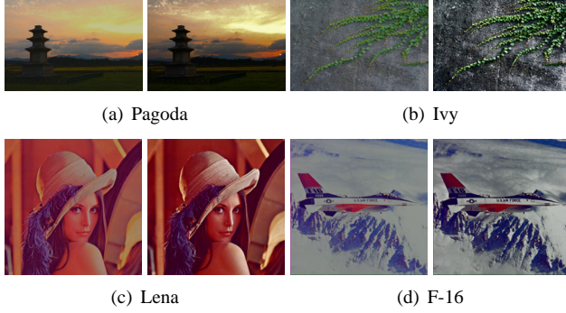
Fig. 1. Comparison of power-reduced output images. In each subfigure, the left image is obtained by the linear mapping method, and the right one by the PCCE algorithm in [5].
