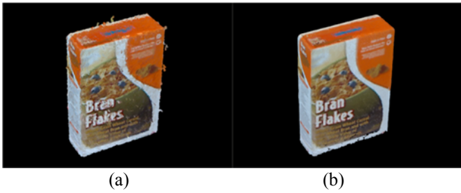
Figure 4. (a) Before 3D de-noising (after registration). (b) After MLS de-noising.
