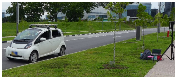
Fig. 4: Experimental setup of the OSA recording using the electric vehicle (EV) with the microphone mounted on top.
