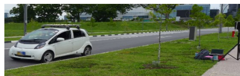
Fig. 3: Experimental setup of the OSA recording using the EV with the microphone mounted on top.
