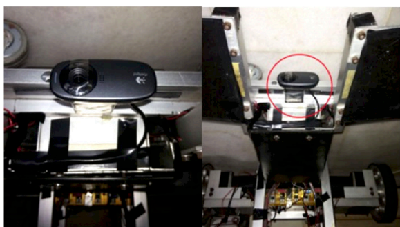
Fig. 3. Mounting of Camera Sensor on Wheelchair. (Left) Front View. (Right) Top View.
