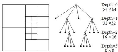
Fig. 1 Flexible quad-tree coding structure of HEVC.
