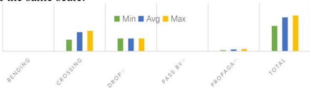
Fig. 18 comparison of insertion loss of ReLONEONoC
