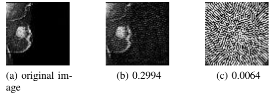
Fig. 2: (a) Original Image. Reconstructed images when (b) Tikhonov regularization and (c) LS are used and the corresponding SSIM.
