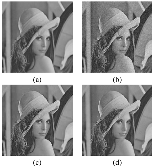
Fig. 2. Watermarked images degraded and distorted through (a) smoothing, (b) adding noise, (c) JPEG compression, and (d) geometric distortion (StirMark)
