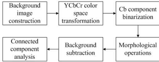
Fig. 1: Block diagram of pre-processing.
