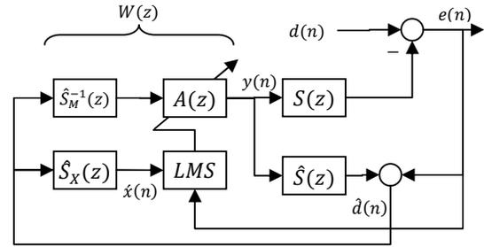
Fig. 3: The proposed structure for adaptive feedback ANC
