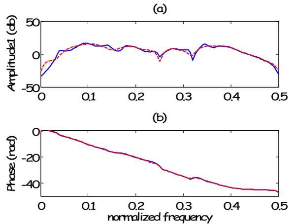
Fig. 4: Frequency response of the secondary path. a) solid: frequency response amplitude of the real system, dashed: frequency response amplitude of the estimated system. b) solid: frequency response phase of the real system, dashed: frequency response phases of the estimated system
