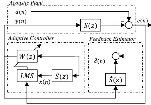
Fig. 2: Available implementation of adaptive feedback ANC
