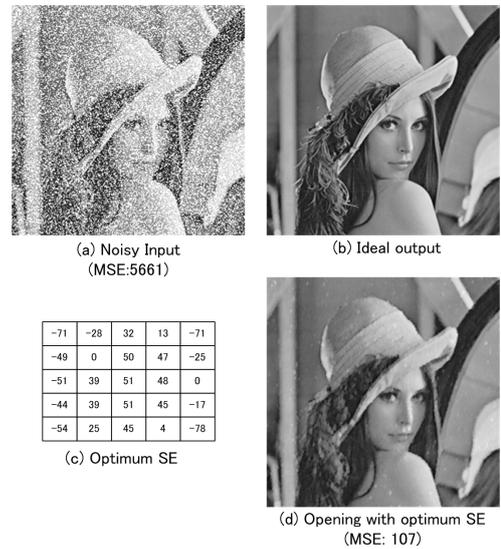
Fig. 4. Design of opening filter for Lenna image.
