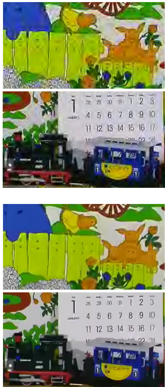
Fig. 8 Compressed Mobile and Calendar image (720x576) at 0.25bpp, by JPEG2000 (top) and the proposed scheme (bottom) respectively. It is observed that the proposed scheme works well on painting, fonts and real-life objects.
