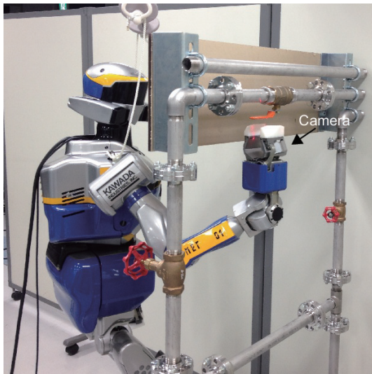
Fig. 1. An example of the tasks for a humanoid robot used in devastated areas. The configuration of the camera mounted on the palm (annotated by "Camera") is shown in Fig. 2. In this figure, microphones are not installed.
