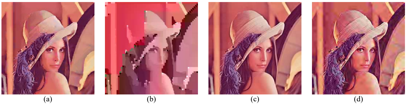
Fig. 14 The visual comparison of the “lena” image under 0.6 bpp. (a) The proposed method. (b) H.264 intra coding (0.8 bpp). (c) JPEG. (d) JPEG2000.
